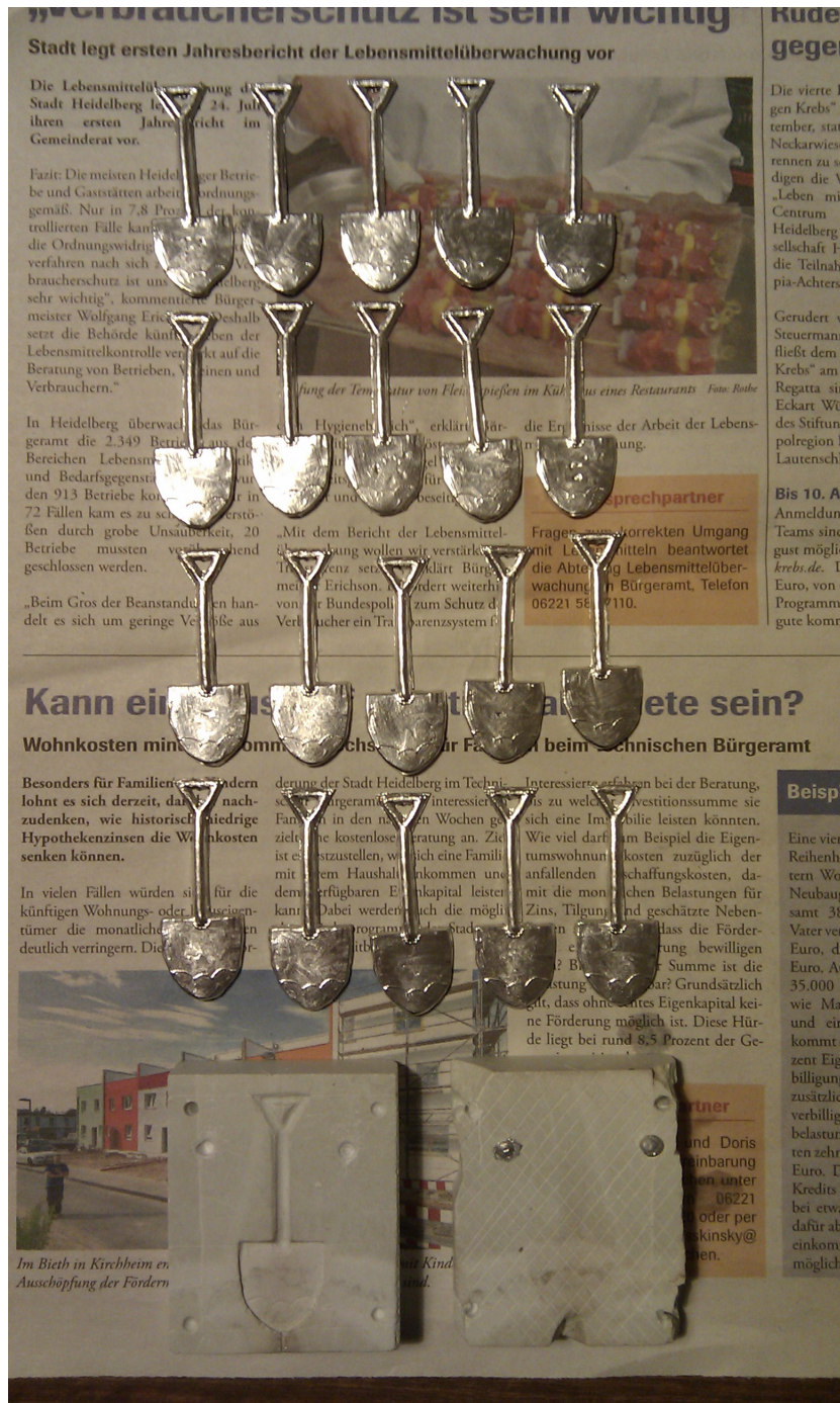
Figure 3: St. Fiacre's Shovels and their mould
